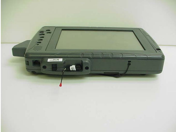
Photograph A.1-1 - Tablet PC in the worst-case Cellular Configuration
