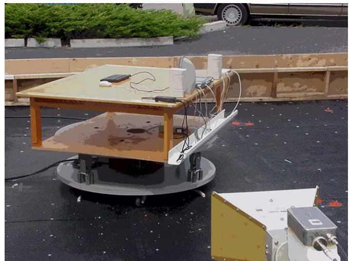
Photograph F.7-2 - Vertical 3115 Horn and LNA Cellular Radiated Emissions Setup
