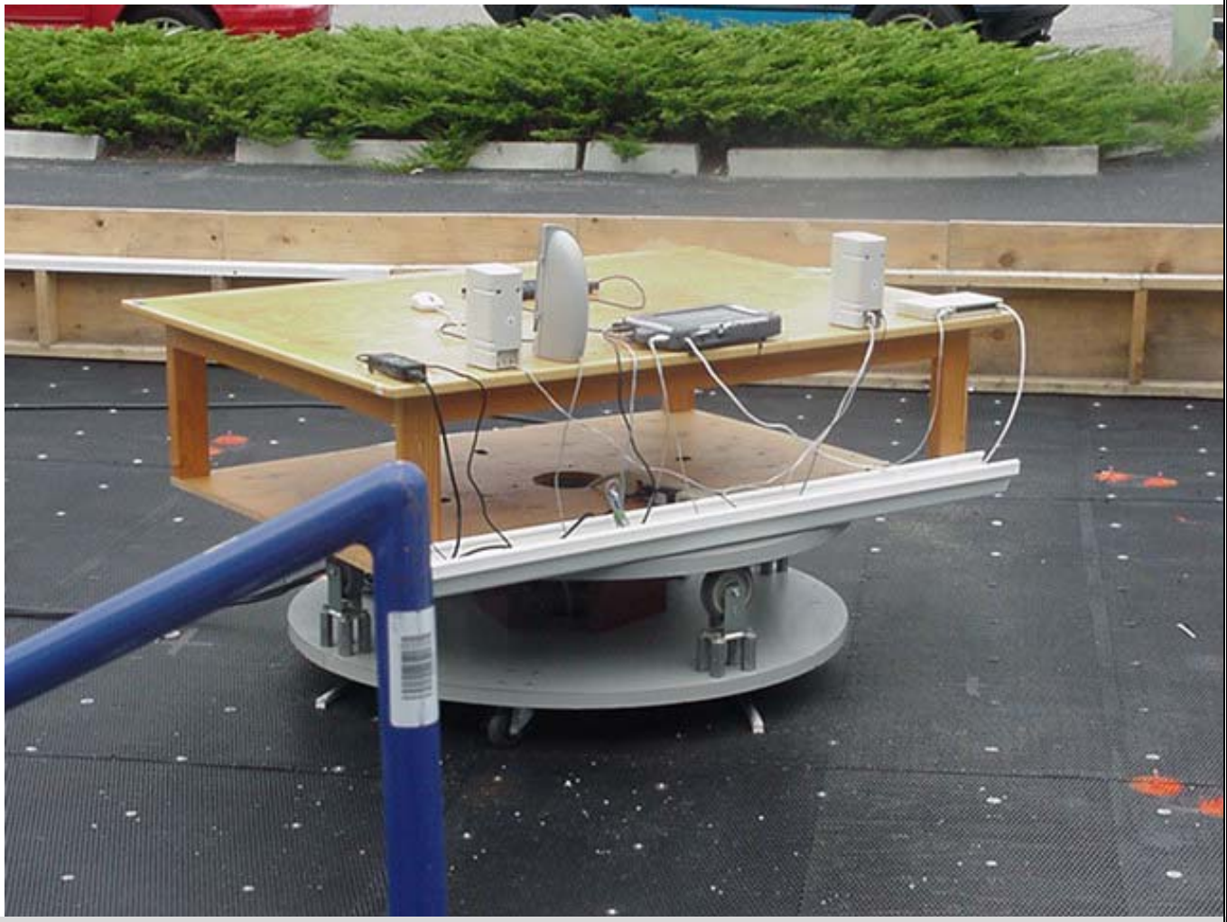
Photograph E.7-1 - DUT in Highest Cellular Carrier Configuration
