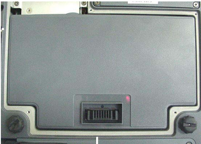
Internal Li-ion Battery 11.1 V, 3600 mAh (Model: T8M-E)
