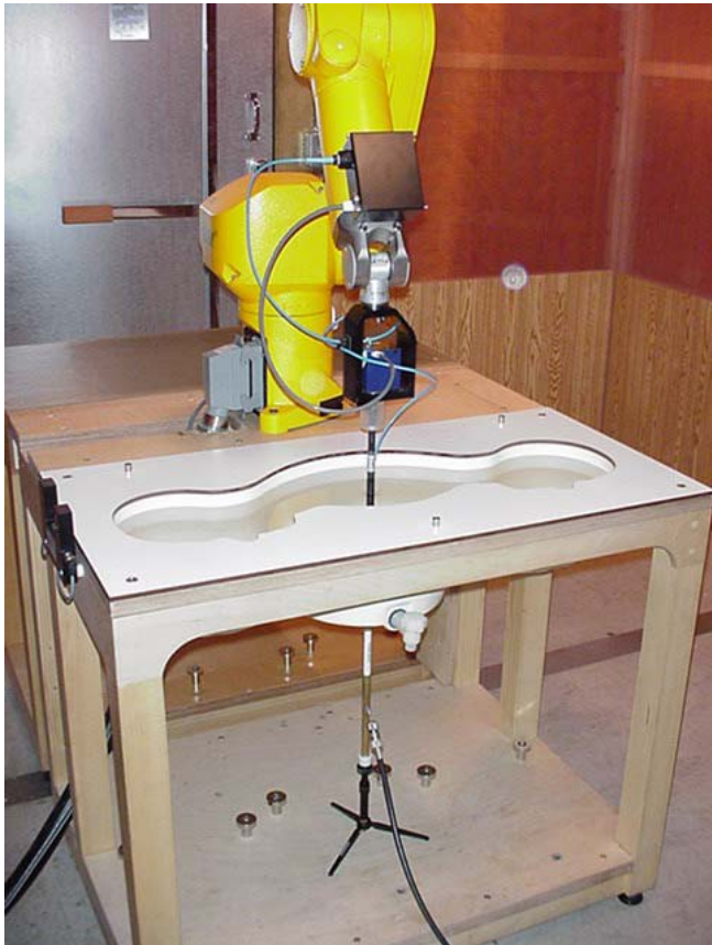
DASY4 SAR Measurement System with SAM phantom
