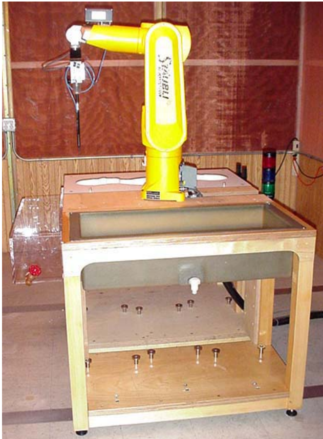
DASY4 SAR Measurement System with planar phantom
