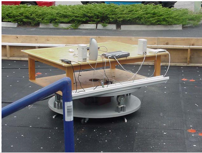
Photograph F.7-1 - Horizontal Bilog Cellular Radiated Emissions Setup
