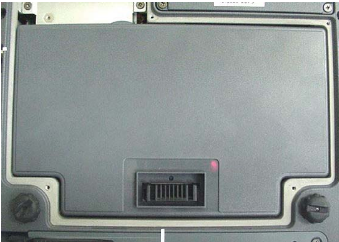
Internal Li-ion Battery 11.1 V, 3600 mAh (Model: T8M-E)
