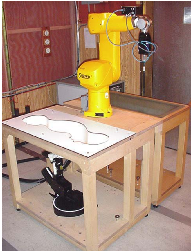
DASY4 SAR Measurement System with SAM phantom
