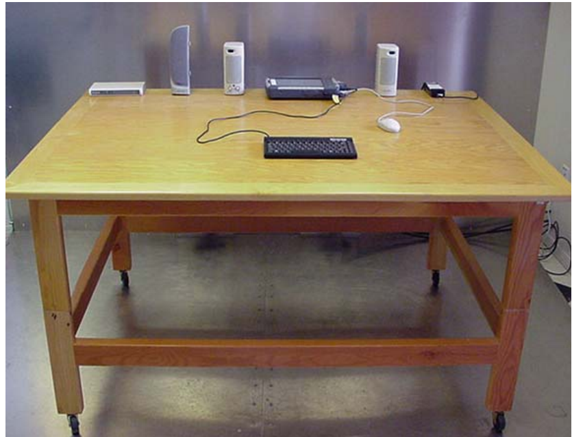
Photograph G-2 - AC Powerline Conducted Emission Configuration
