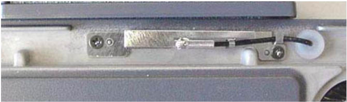
WLAN Antenna 2 (Transmit / Receive)
