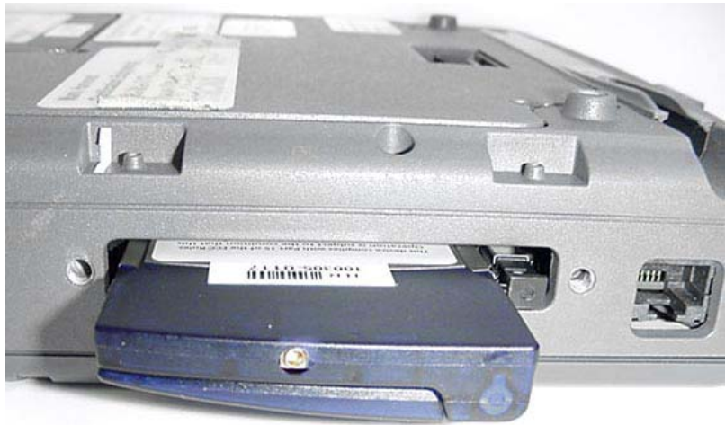
AirCard 580 installed in IX325 PCMCIA Slot (Broadband Hatch & Antenna Removed)
