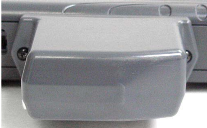
IX325 Broadband Hatch (AirCard 580 Antenna Removed)
