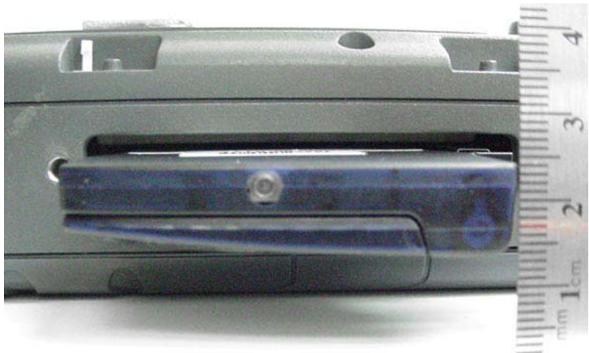
AirCard 580 Card-to-Base Distance (Broadband Hatch & Antenna Removed)
