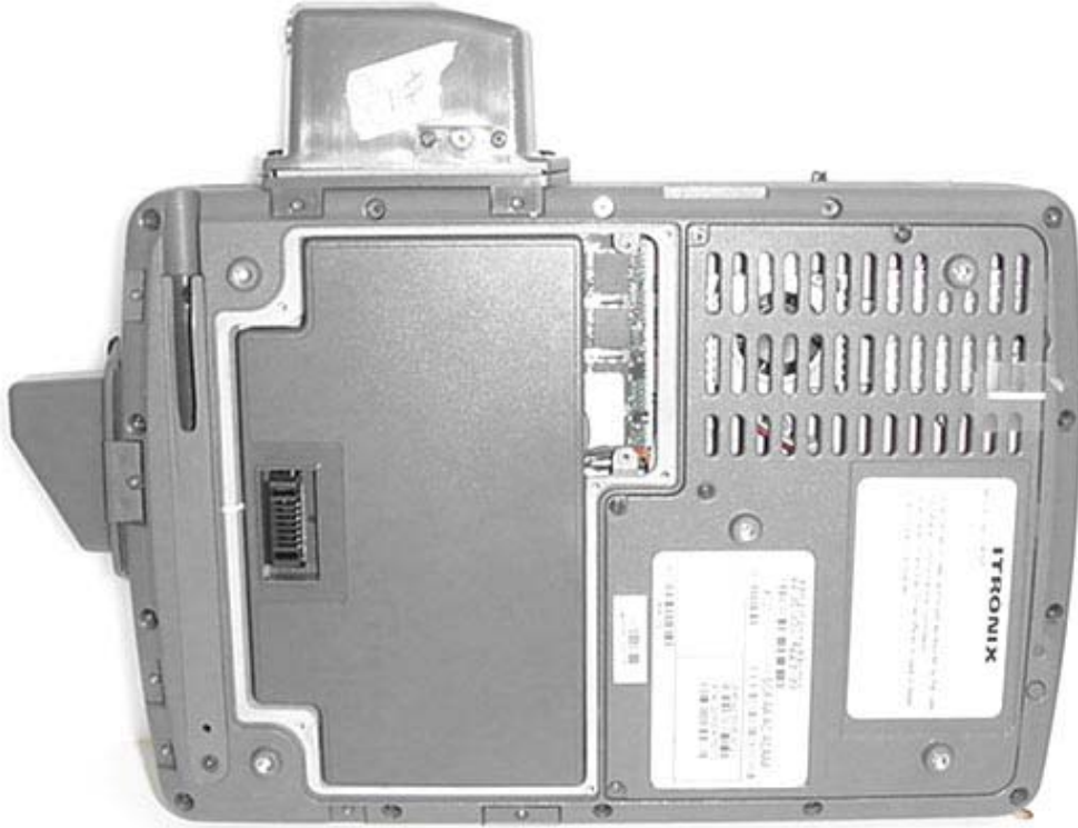
IX325 with Internal Lithium-ion Battery (Model: T8M-E)
