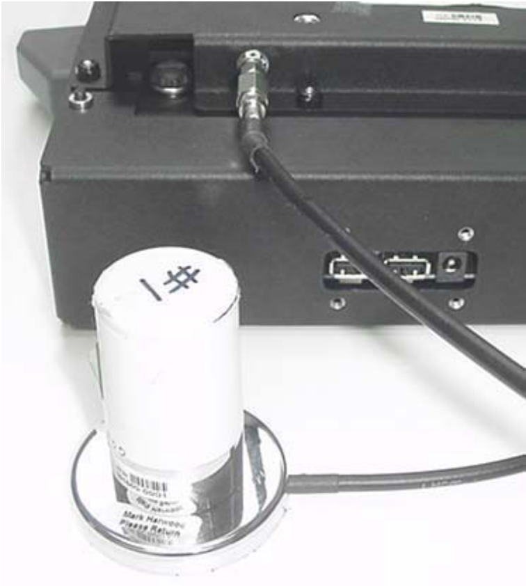
MaxRad 3dBi Antenna connected to IX325 Vehicle Dock
