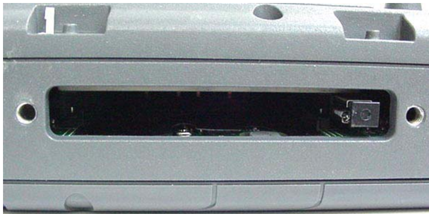
IX325 PCMCIA Card Slot (AirCard 580 Removed)
