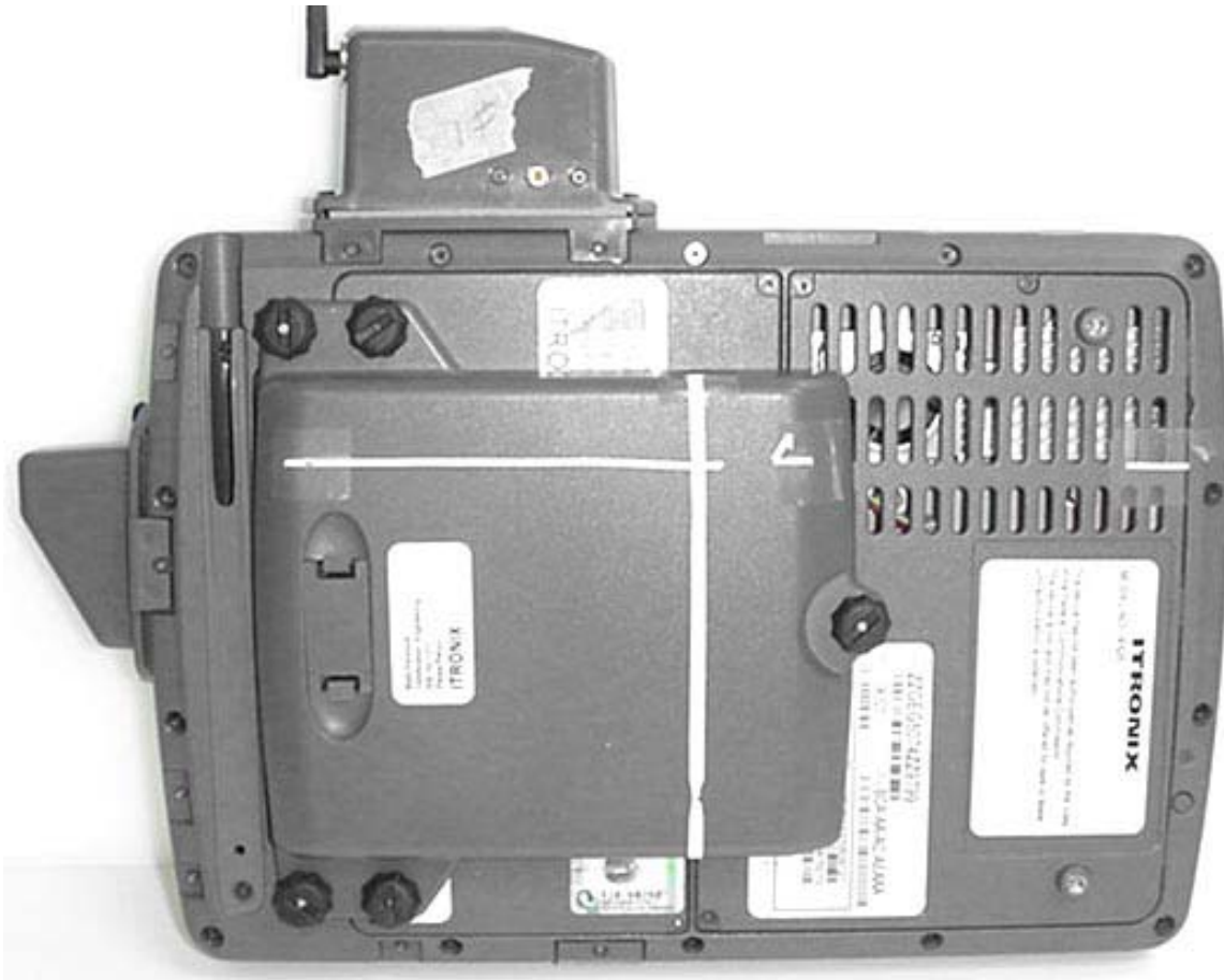
IX325 with External Second Lithium-ion Battery (Model: T8S-E)
