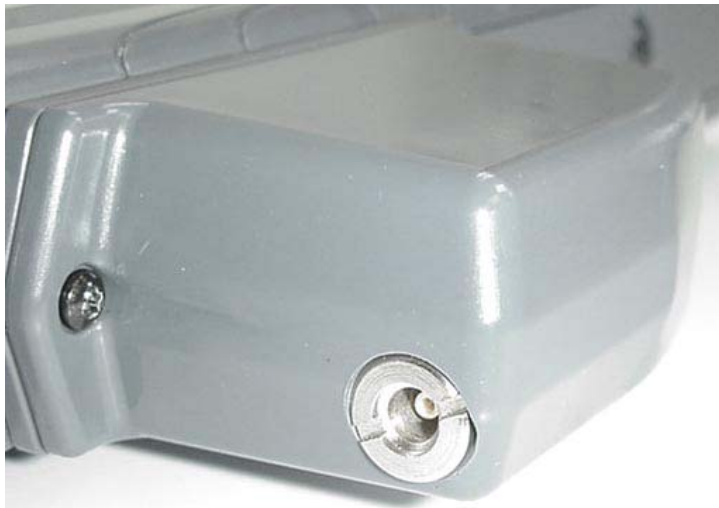
IX325 Broadband Hatch (AirCard 580 Antenna Connector)
