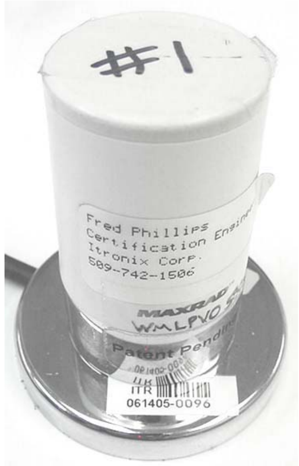
MaxRad 3dBi Vehicle Antenna (P/N: WMLPVDB800/1900)
