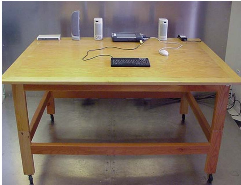
Photograph G-2 - AC Powerline Conducted Emission Configuration
