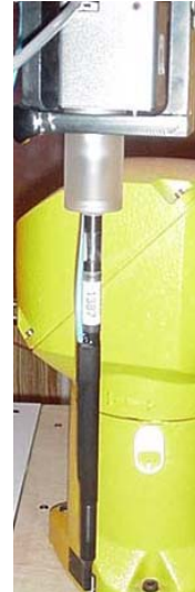
ET3DV6 E-Field Probe
