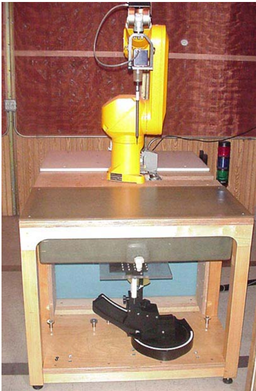
DASY4 SAR Measurement System with planar phantom
