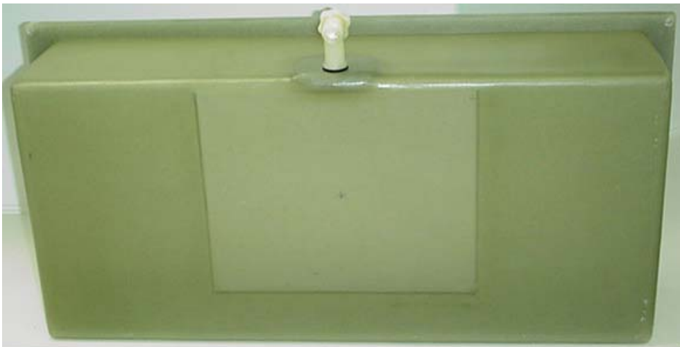
Fiberglass Planar Phantom - Bottom View
