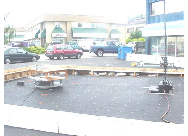
Photograph I.8-6 - 3160-09 Horn (18GHz - 24GHz)
