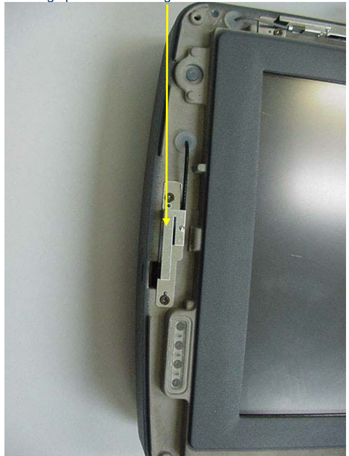
Photograph A.1-6 - Left Edge Bluetooth Antenna Location
