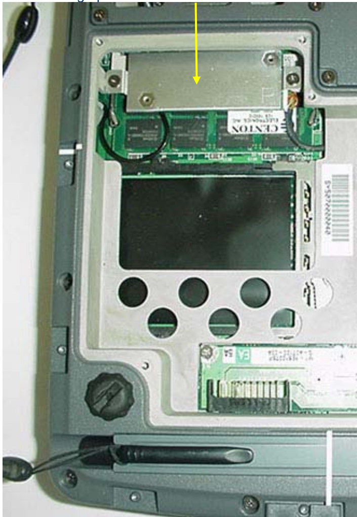
Photograph A.1-5 - Internal Bluetooth Location
