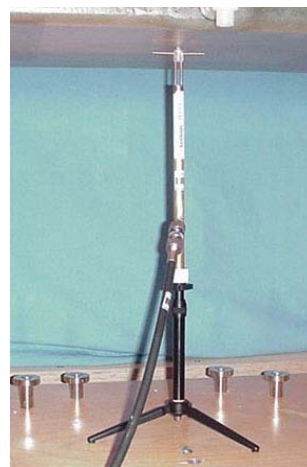
1900MHz Dipole Setup
