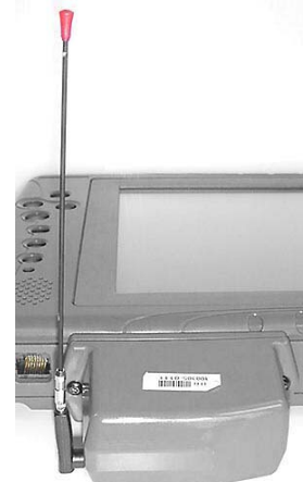
Antenna "Perpendicular" ("0 Degrees Landscape" Device User Orientation)
