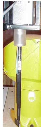
ET3DV6 E-Field Probe
