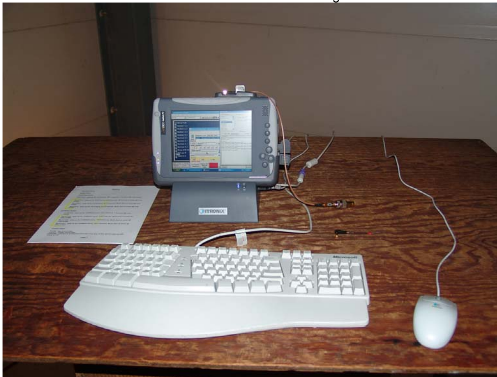
AirCard 775 antenna removed and a resistive 50 ohm load connected during the radiated spurious and harmonics measurements.
