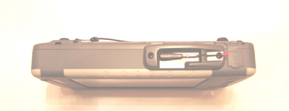
'Top View IX300 AC775 Antenna visible
