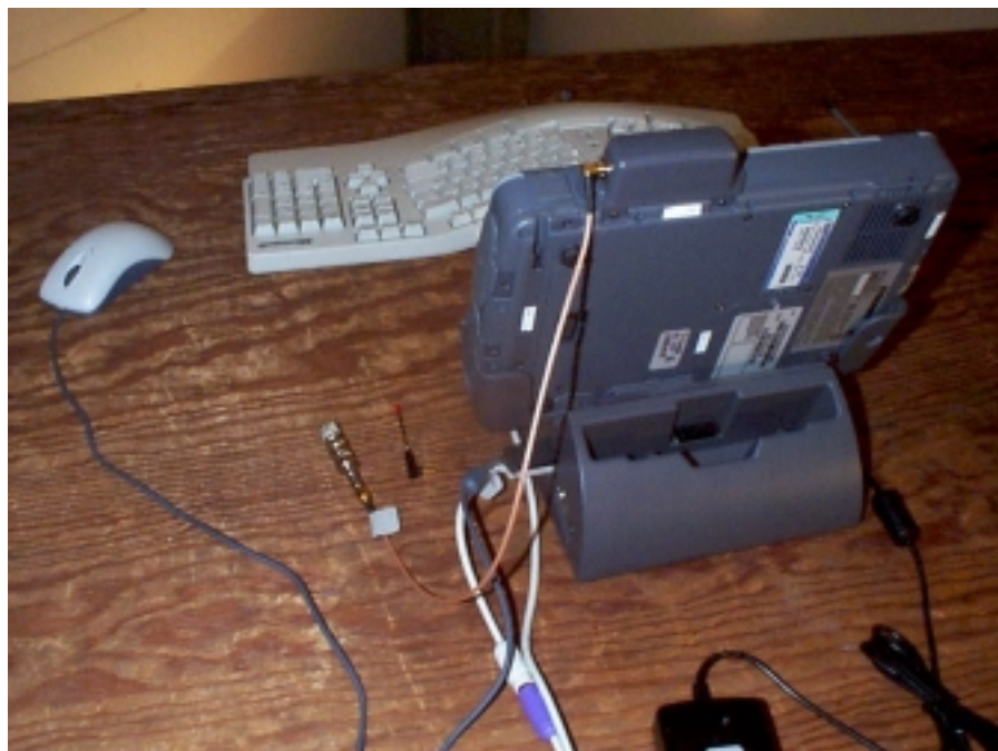
AirCard 750 antenna removed and a resistive 50 ohm load connected during the radiated spurious and harmonics.
