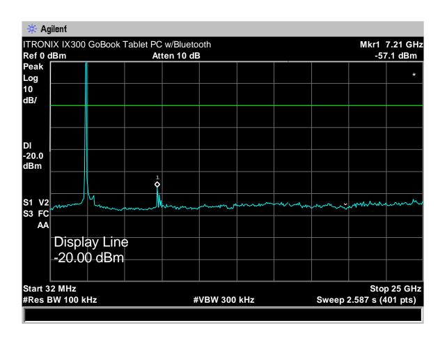
Plot 10 - Lower Band-edge Compliance of RF Conducted Emissions
