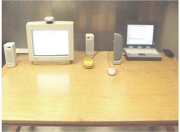
Photograph G-2 - AC Powerline Conducted Emission Cable Placement
