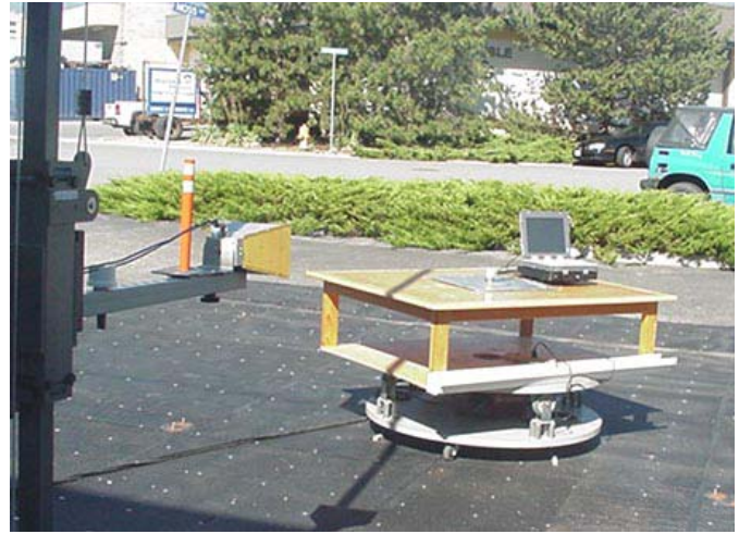
Photograph B.7-6 - Horn Receive Antenna with DUT Vehicle-Mount Antenna Configuration
