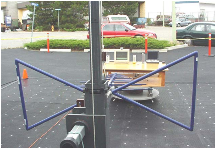
Photograph F-3 - Front of Radiated Emission Configuration
