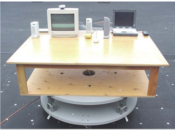
Photograph F-3 - Front of Radiated Emission Configuration
