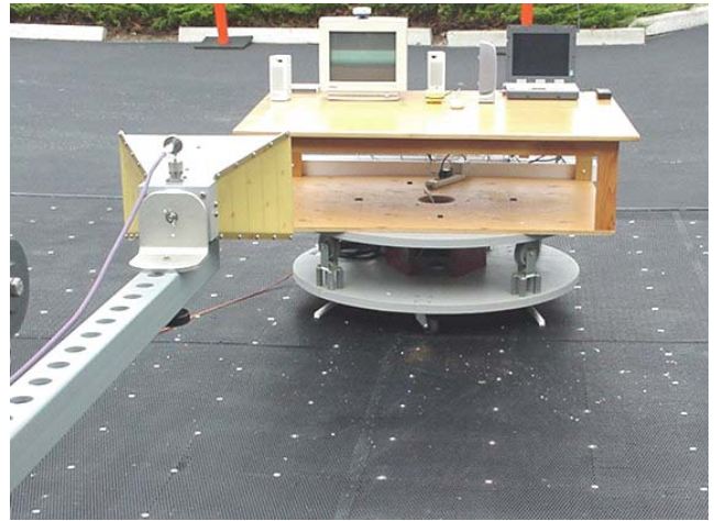
Photograph F-4 - Back of Radiated Emission Configuration
