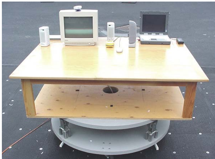
Photograph E-3 - Front of Radiated Emission Configuration
