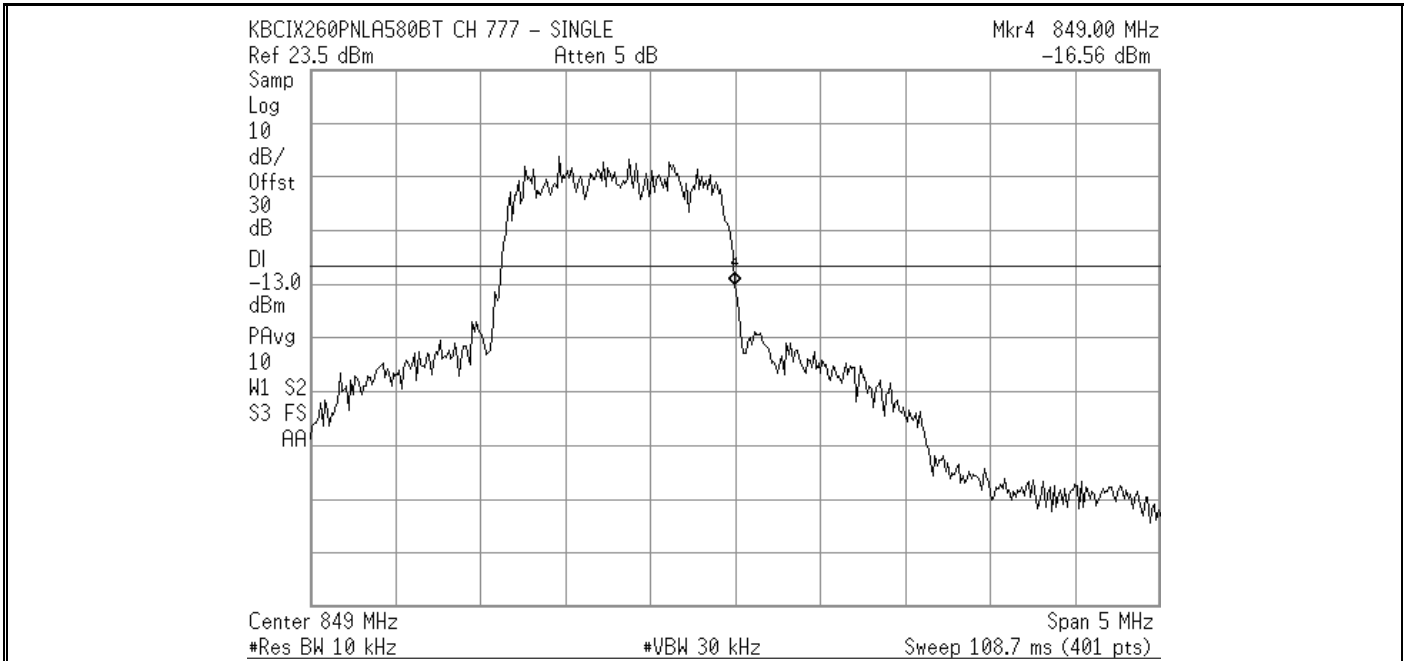
Figure C.8-4 - Channel 777 (848.31 MHz) Upper Cellular CDMA Band-edge at 849.0 MHz
