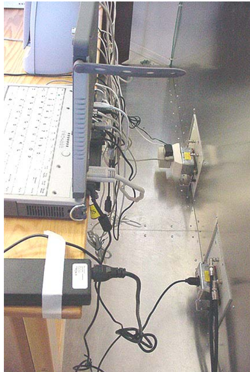
Photograph H-2 – AC Powerline Conducted Emission Cable Placement
