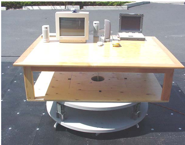
Photograph E-3 - Front of Radiated Emission Configuration
