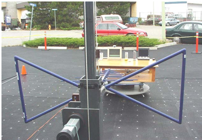
Photograph F-3 - Front of Radiated Emission Configuration
