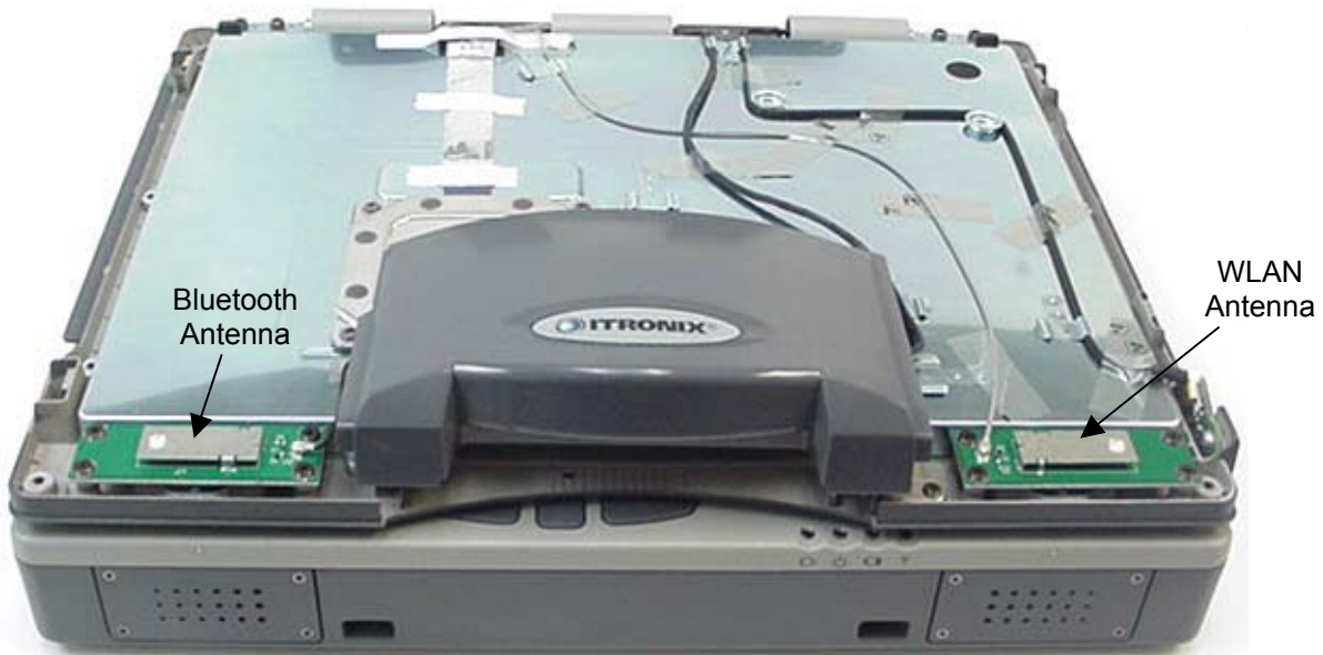
Photograph A-7 - Surface Mount Antenna Placement
