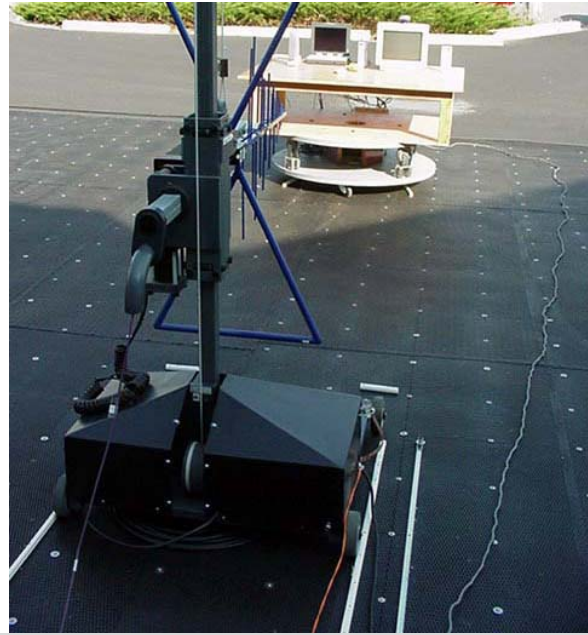
Photograph D-4 - Back of Radiated Emission Configuration
