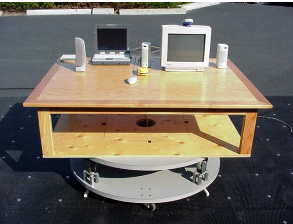
Photograph D-3 - Front of Radiated Emission Configuration
