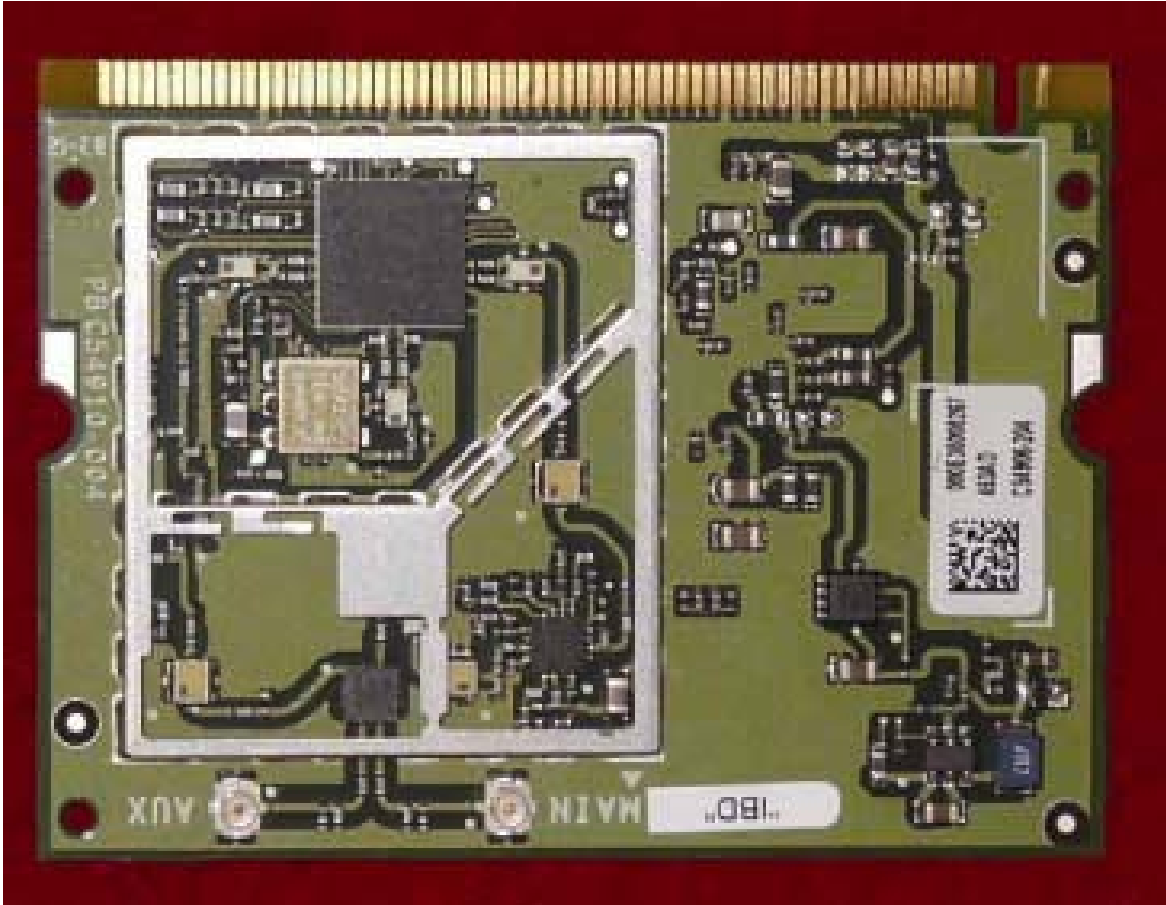
Front with Shielding Removed
