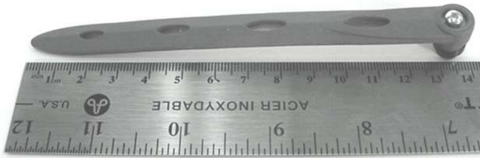
Dual-Band GSM External Swivel Dipole Antenna
