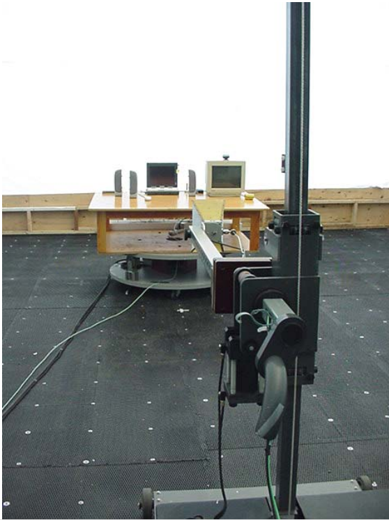
Photograph E.7-1 - Horizontal Horn Receive Antenna with DUT
