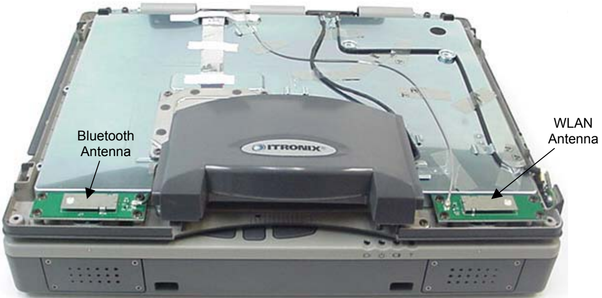
Photograph A-7 - Surface Mount Antenna Placement
