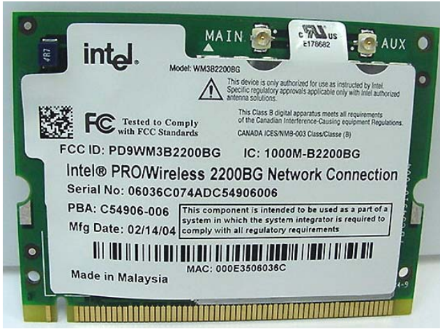
Photograph A-5 - WLAN Mini-PCI Card
