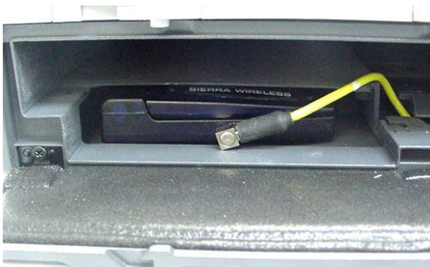
Photograph A.1-7 - CDMA Modem installed in PC
