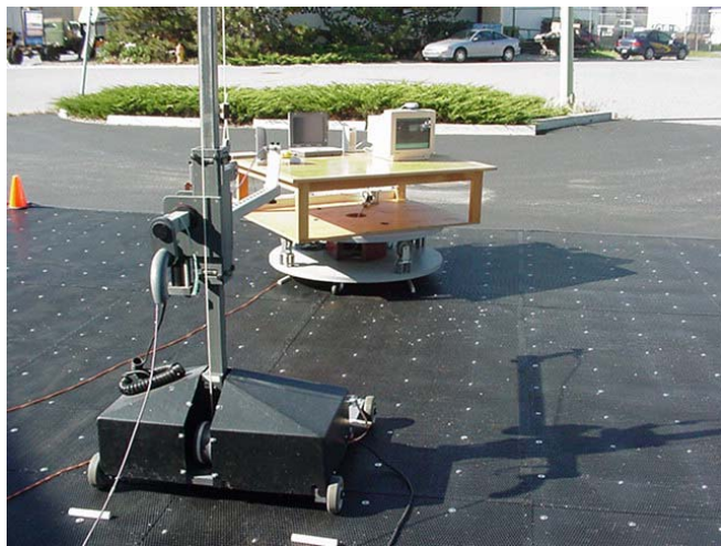
Photograph H-2 - 3160-09 Horn Antenna (18-26GHz)
