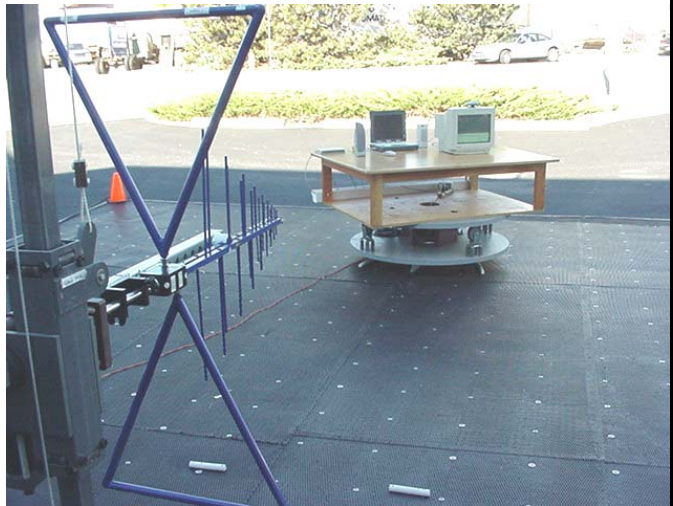
Photograph I-4 - Vertical Polarization (30MHz - 1 GHz)
