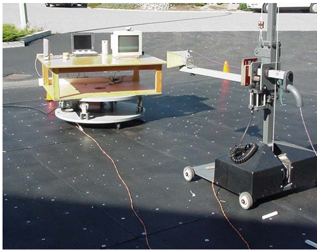
Photograph H-1 - 3115 Horn Antenna (1-18GHz)
