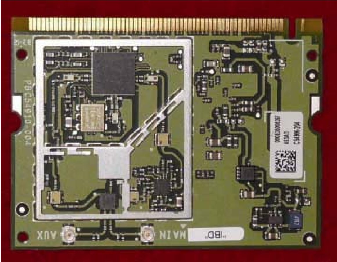
Front with Shielding Removed
