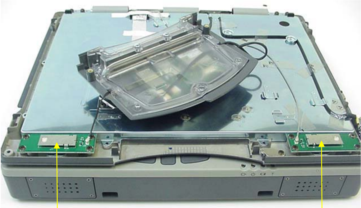
Bluetooth Surface-Mount Antenna (Upper Rear Left Side Edge of LCD Display)
