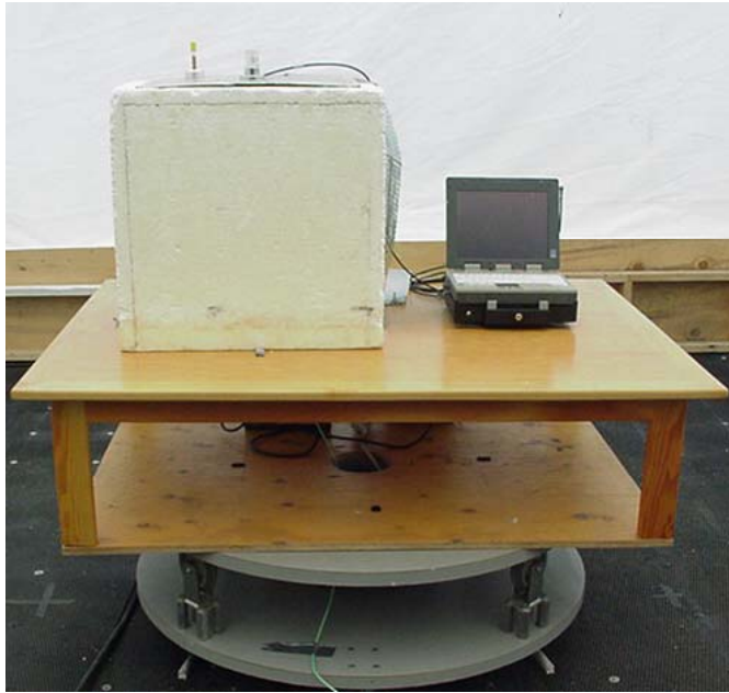
Photograph F.7-5 - Front of Radiated Emission Setup with vehicle-mount antenna and cradle
