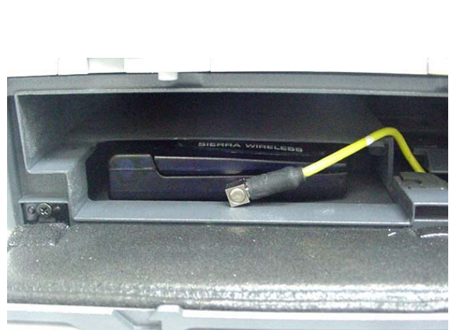
Photograph A.1-6 - CDMA Modem installed in DUT
