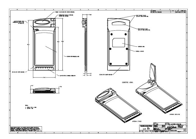
Figure 1: PC3220 PC Card Mechanical Drawing
