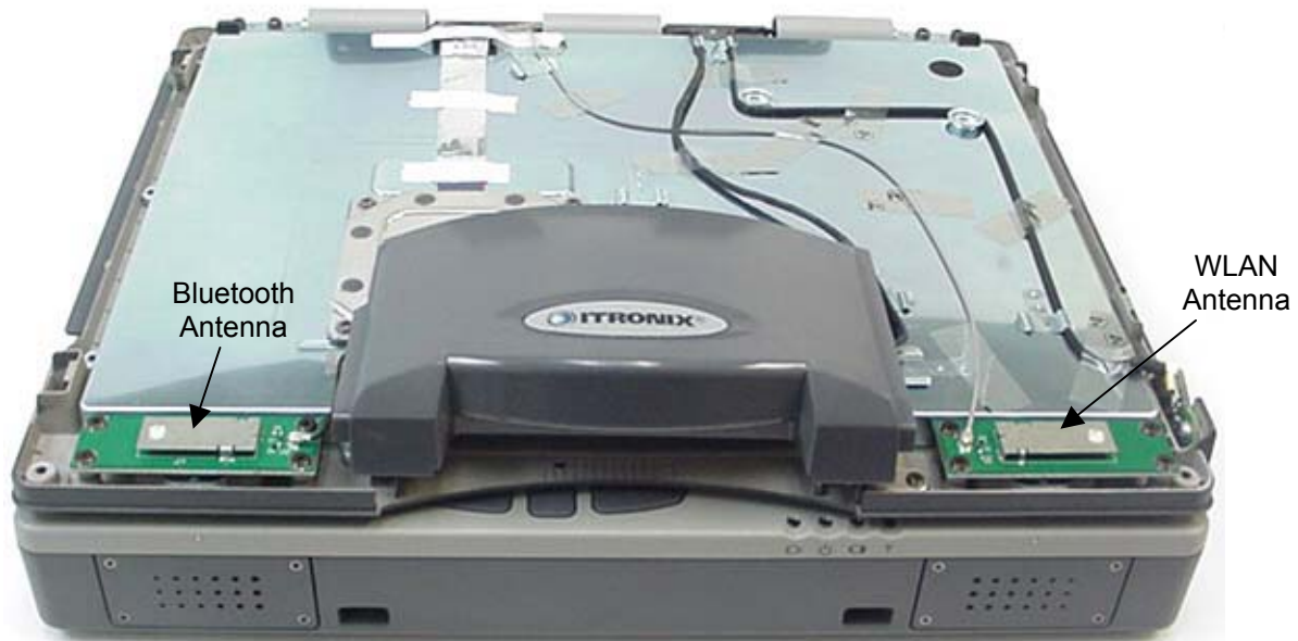
Photograph A-7 – Surface Mount Antenna Placement
