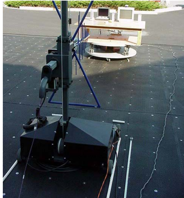
Photograph D-4- Back of Radiated Emission Configuration
