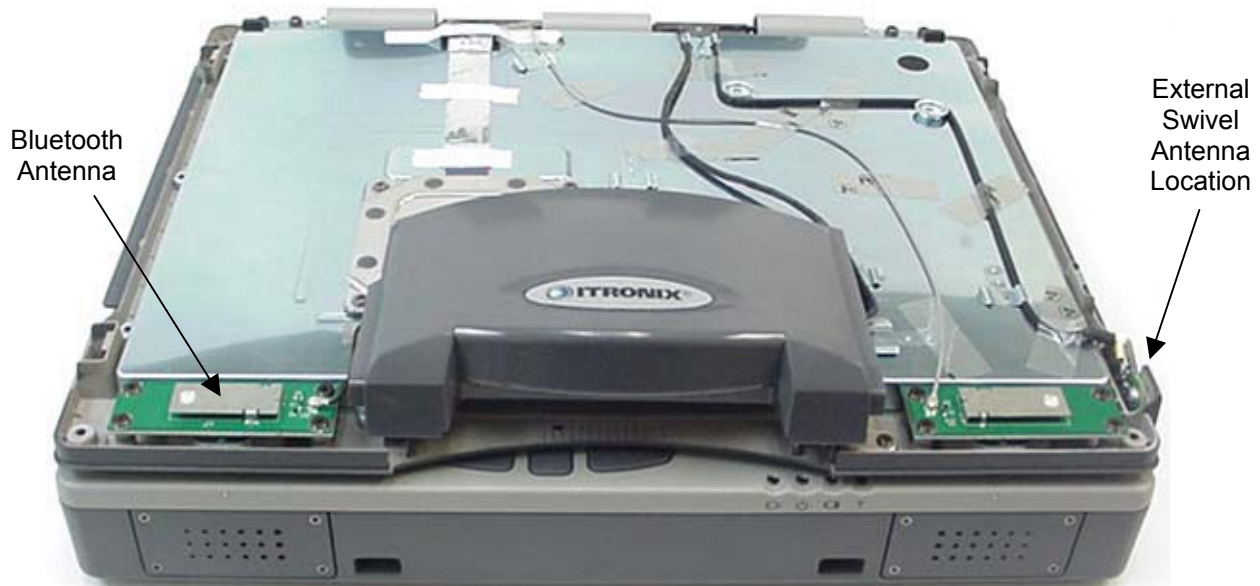
Photograph A-7 – Surface-Mount Antenna Placement
