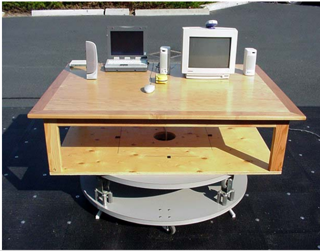
Photograph I-5 - Front of Radiated Emission Configuration
