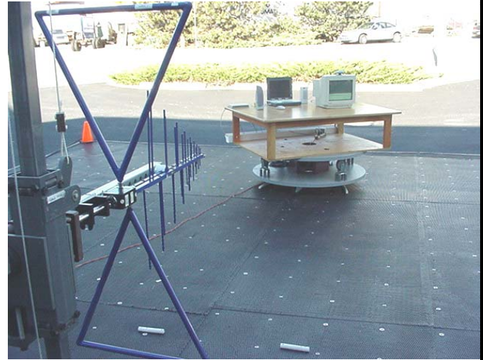
Photograph I-4 - Vertical Polarization (30MHz – 1 GHz)
