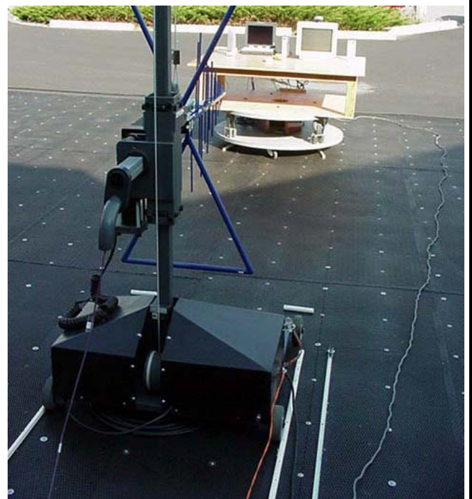
Photograph I-4 - Vertical Polarization (30MHz – 1 GHz)
