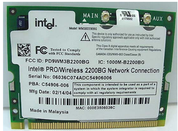
Photograph A-11 - Front of Intel Pro 2200BG Mini-PCI WLAN Card
