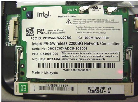
Photograph A-10 - Front of Intel Pro 2200BG Mini-PCI WLAN Card in IX260+ Laptop PC
