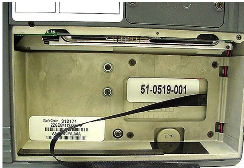
Photograph A-8 - Battery Compartment of IX260+ Laptop PC
