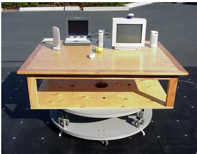
Photograph F-3 - Front of Radiated Emission Configuration
