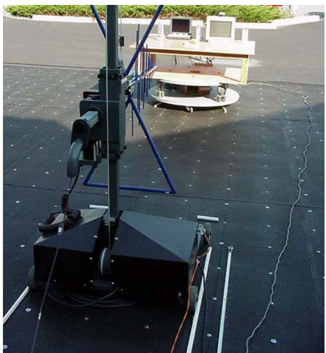
Photograph F-4 - Back of Radiated Emission Configuration
