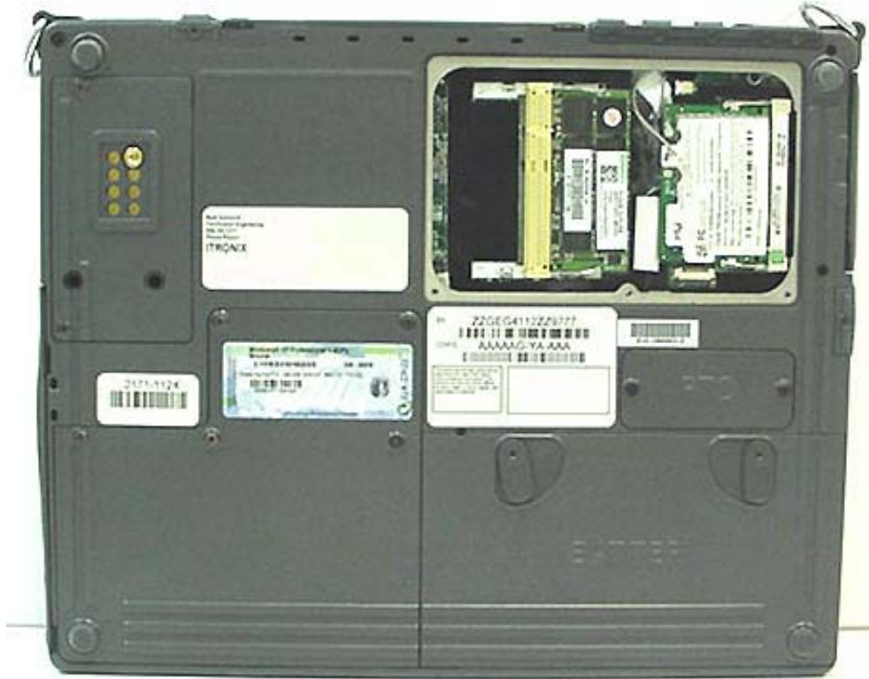
Photograph A-10 - Front of Intel Pro 2200BG Mini-PCI WLAN Card in IX260+ Laptop PC
