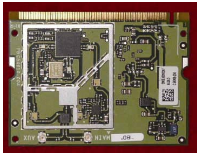
Photograph A-14 - Front of Intel Pro 2200BG Mini-PCI WLAN Card with Shielding Removed
