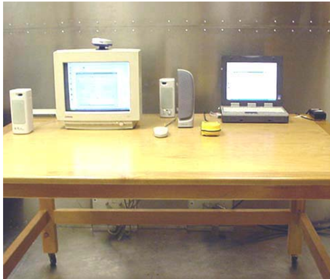
Photograph H-1 – AC Powerline Conducted Emission Configuration
