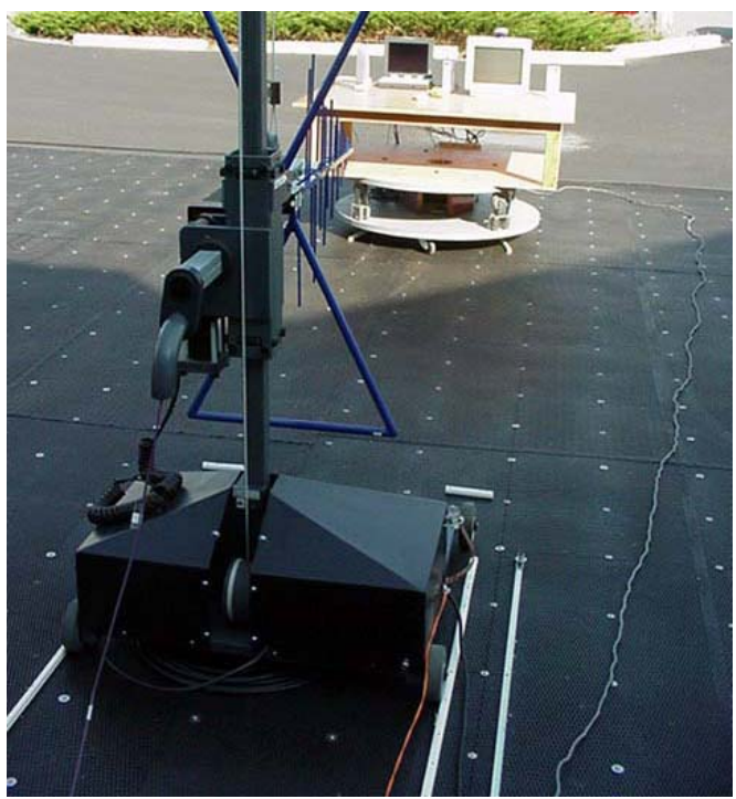
Photograph E-4 - Back of Radiated Emission Configuration
