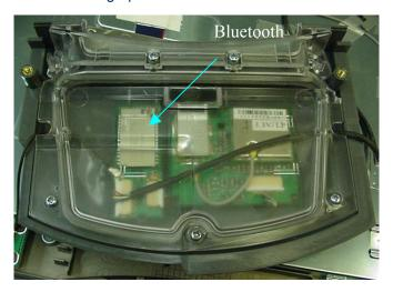
Photograph A-7 - Surface Mount Antenna Placement
