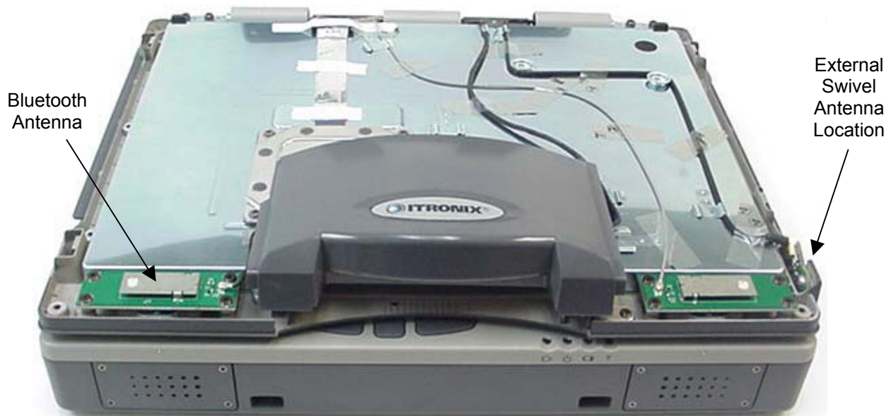
Photograph A-7 - Surface-Mount Antenna Placement
