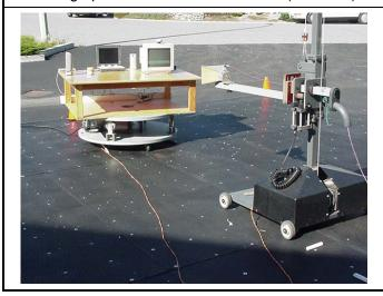
Photograph H-2 - 3160-09 Horn Antenna (18-26GHz)
