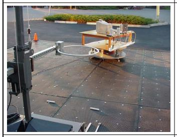
Photograph I-2 - Bilog Antenna (30MHz - 1 GHz)
