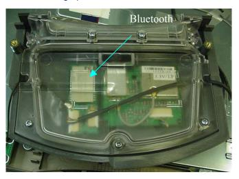
Photograph A-7 - Surface-Mount Antenna Placement
