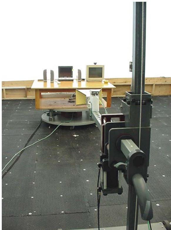
Photograph F.7-4 - Front of Radiated Emission Setup with vehicle-mount antenna and cradle
