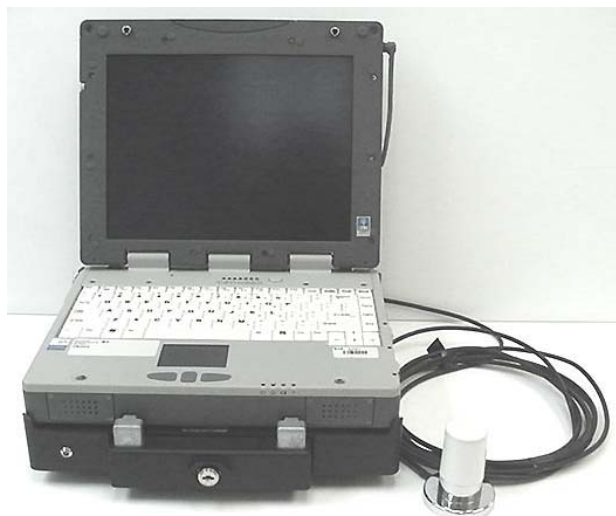
Photograph A.1-3 - DUT in Vehicle Cradle with Vehicle-Mount Antenna - front
