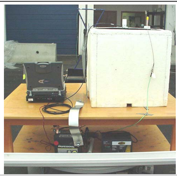
Photograph C.7-6 - Back of Radiated Emissions Setup with vehicle-mount antenna and cradle
