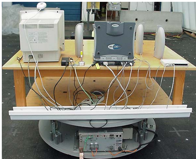
Photograph F.7-3 - Back of Radiated Emission Setup with attached swivel dipole antenna
