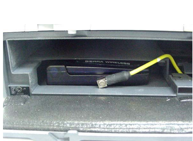
Photograph A.1-6 - CDMA Modem installed in DUT
