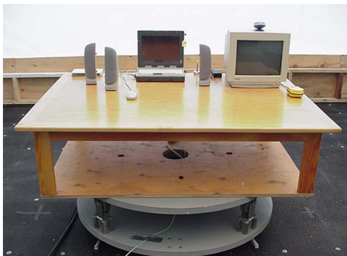
Photograph E.7-3 - Front of Radiated Emission Setup with attached swivel dipole antenna
