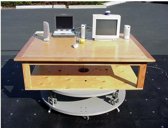
Photograph F-2 - Front of Radiated Emission Configuration
