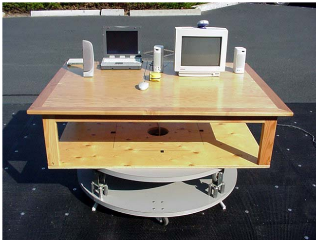
Photograph F-2 - Front of Radiated Emission Configuration
