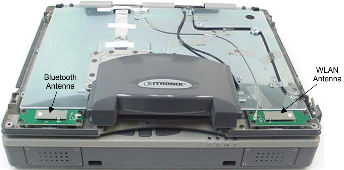
Photograph A-7 - Surface Mount Antenna Placement
