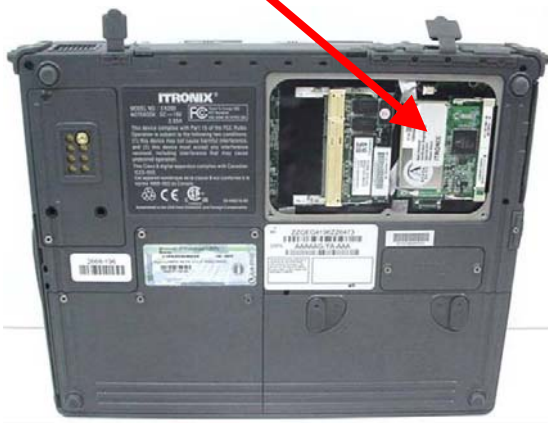
Photograph A-3 - WLAN Mini-PCI Card Location
