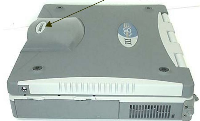
Photograph A-4 - Bluetooth Transmitter Location
