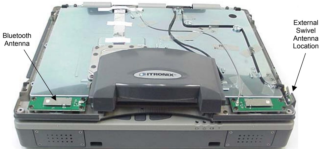
Photograph A-7 - Surface-Mount Antenna Placement
