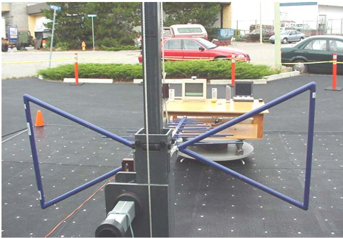
Photograph F-3 - Front of Radiated Emission Configuration
