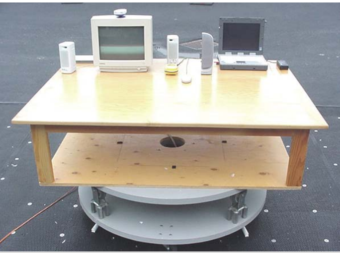
Photograph F-3 - Front of Radiated Emission Configuration
