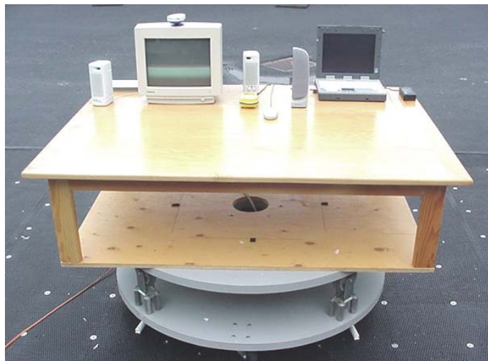
Photograph E-3 - Front of Radiated Emission Configuration
