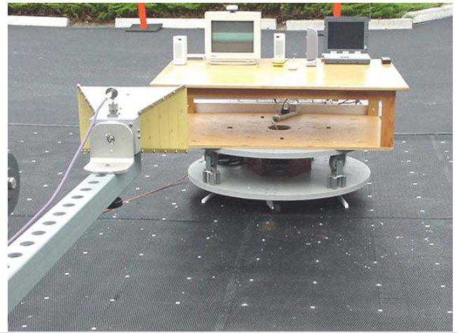
Photograph F-4 - Back of Radiated Emission Configuration
