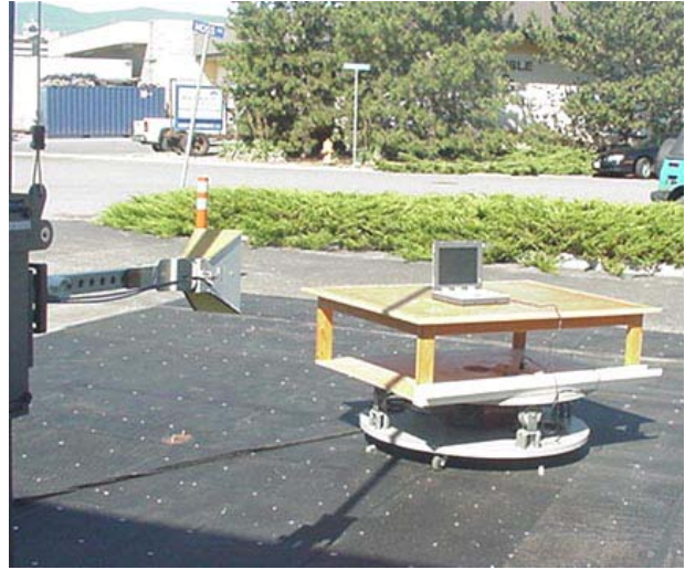
Photograph B.7-4 - Horn Substitution Setup
