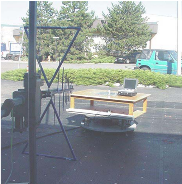
Photograph B.7-7 - Dipole Substitution Setup
