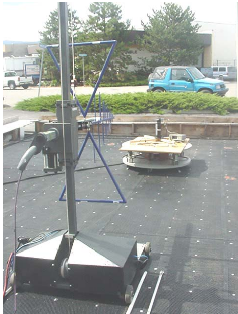
Photograph B.7-7 - Dipole Substitution Setup
