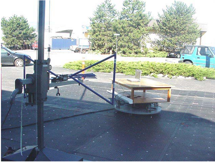
Photograph B.7-3 - Dipole Substitution Setup
