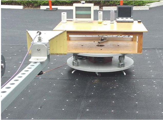
Photograph E-3 - Front of Radiated Emission Configuration
