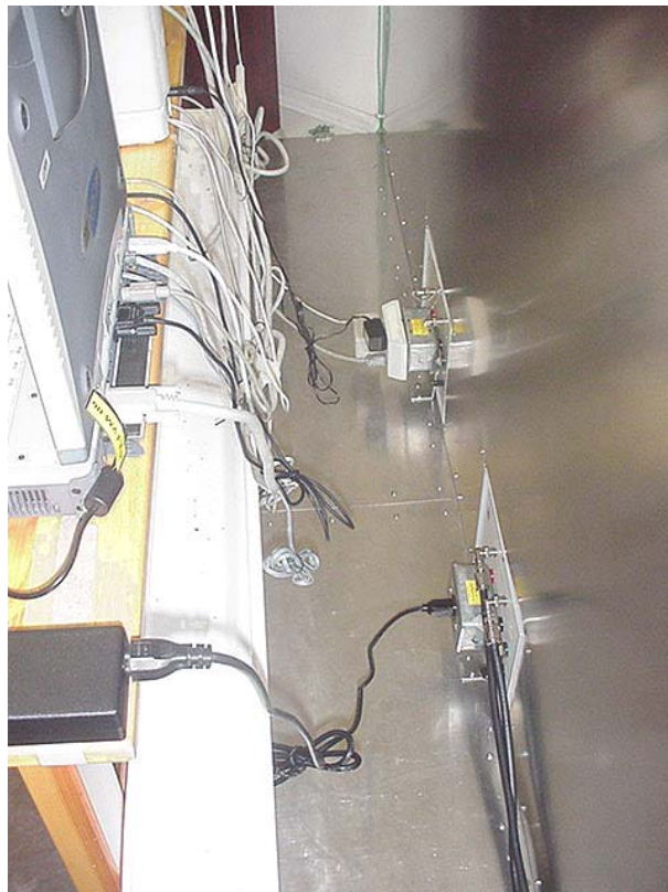
Photograph H-2 - AC Powerline Conducted Emission Cable Placement
