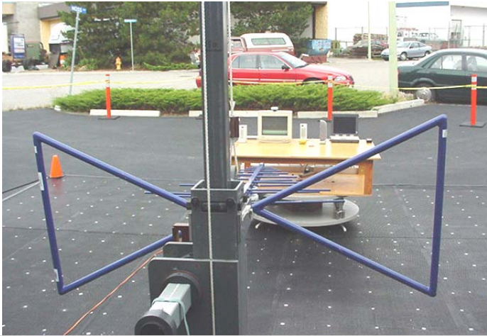
Photograph F-3 - Front of Radiated Emission Configuration
