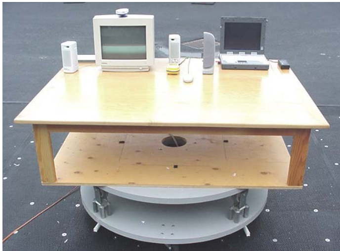
Photograph E-3 - Front of Radiated Emission Configuration
